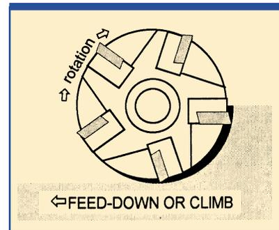
*direction* as the feed. The insert enters through the unmilled surface and produces a chip that becomes progressively thinner as the insert passes through the part.
