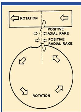
**Double Positive** for milling cutters uses conventional positive rake insert geometries, this style of cutter is used where freer cutting action and lower cutting pressures are required. These cutters also produce a good work piece finish and often reduce workpiece deflection and vibration.
