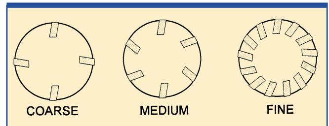
**Coarse pitch** cutters are used for general purpose and heavy chip load milling operations. They have large chip gullets and adequate clearances to accept large depths of cut and high feed rates. **Coarse pitch** cutters generally draw less horsepower owing to fewer inserts engaged in cutting simultaneously.
