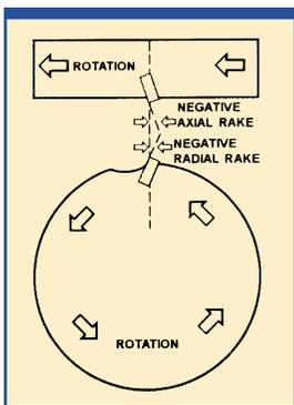
**Double Negative** rake cutters use conventional negative rake insert geometries. This style of cutter is used for maximum insert economy and in heavy-duty applications where adequate horsepower is available to handle the higher chip loads that are generated.
