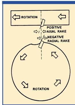
**Negative-Positive** rake angle cutters frequently use a negative rake insert to achieve negative radial geometry but have a positive relief angle ground under faceted corners to achieve a positive axial geometry. This style of cutter combines high insert strength with reduced cutting pressures. They are
