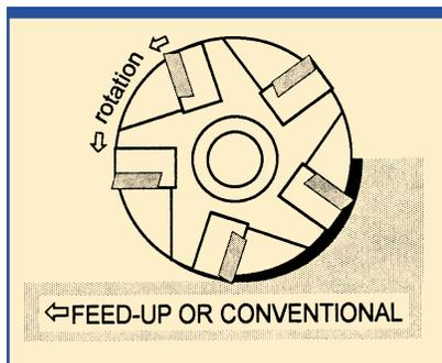
unmilled surface. This may be of advantage if the surface has heavy scale. On the other hand, **up milling** tends to lift the work piece during the cut. It can also result in work hardening at the milled surface on certain materials.
