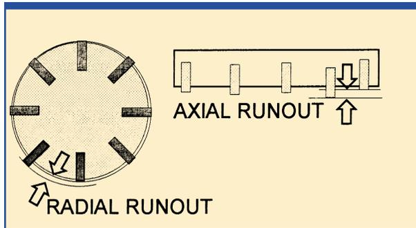
**Fixed pocket milling cutters** have no means of compensating for runout caused by manufacturing tolerances of inserts and cutter bodies. Therefore, there are several steps necessary to minimize the adverse effects of runout.
