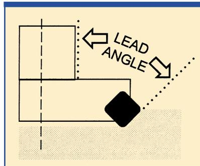
Where a square shoulder is necessary on the part, use a 0-degree lead angle. Triangle or parallelogram inserts must be used to provide for end clearance on the cutter. If the
